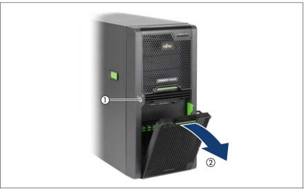
Figure 23: Removing the hard disk cover
